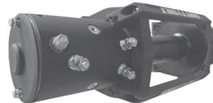
**Step 5:** Re-install the 2 long bolt on the motor end cap
