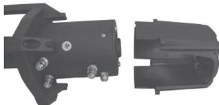
**Step 2:** Remove the motor cover
