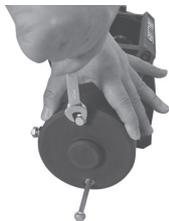
**Step 3:** Loosen and remove the 2 long bolts on the motor end cap
