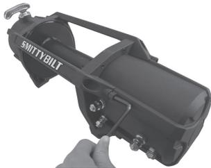
**Step 1:** Loosen and remove the 4 motor bracket bolts
