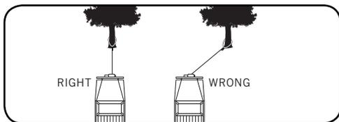
Short pulls from an angle can be used to straighten the vehicle. Long pulls should be done with the wire rope at a 90° angle to the winch/vehicle.
