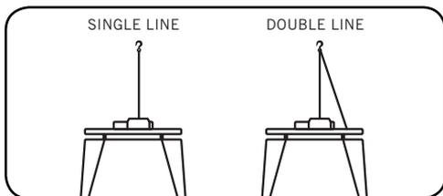
This reduces the load on the winch and the strain on the rope by approximately 50%.
