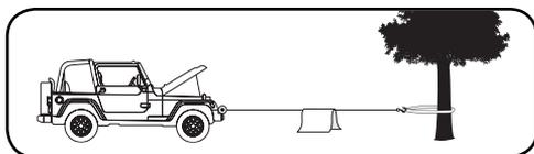
In the event of a broken cable it will dampen the snap back. For additional protection open the hood of the vehicle. For pulls over 8,000 lbs., we recommend the use of the snatch block/pulley block to double line the wire rope.
